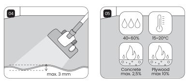
If the first three points are not met, this can be remedied by applying a primer onto your surface. A primer provides the screed with a top layer and reinforces it. If the surface is not level enough, you can level it. Get information from a good adhesive manufacturer for the use of the correct preparation products.
